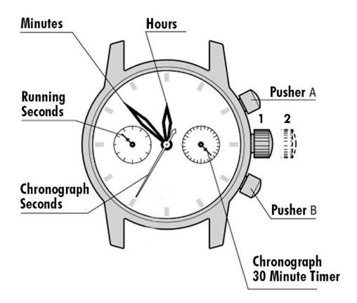
**To set the time:** Pull out the crown from position 1 to 2. Rotate the crown until you
